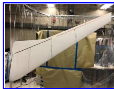
Fig. 4. Copper tape electrode placed near trailing edge on the upper surface of the CRM-NLF.
