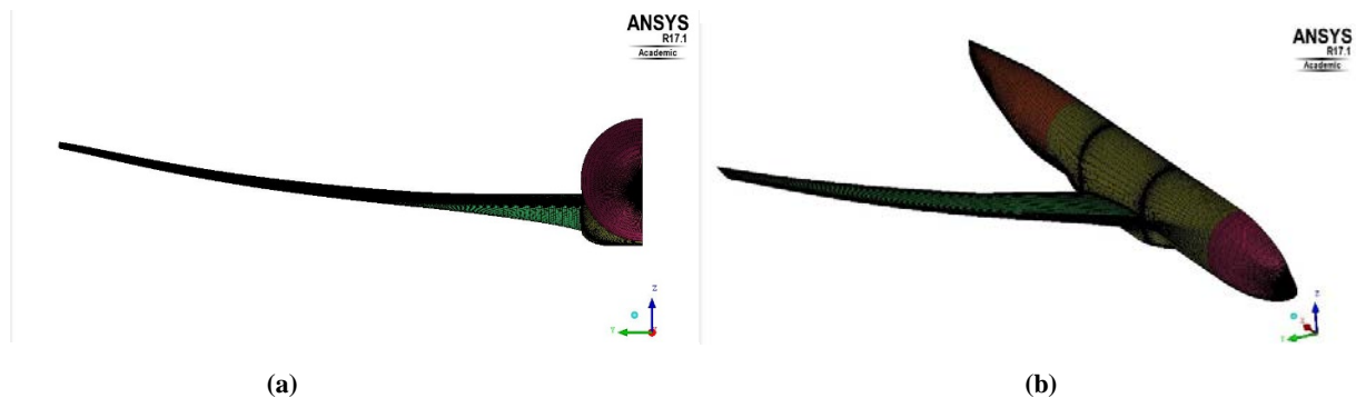
Figure 20 Aero-elastic geometry of WB and surface mesh
