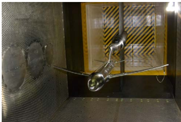
Figure 2. The 80% scaled NASA CRM model installed in the test section.
