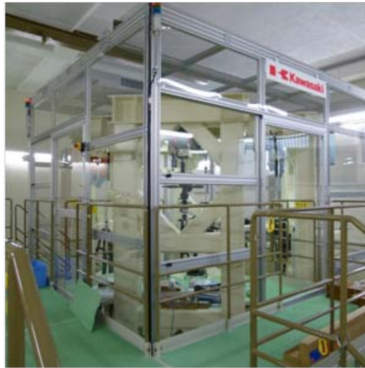
Figure 3. JAXA automatic balance calibration machine.
