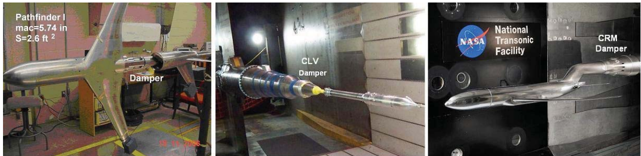
Figure 14: Models and Active Sting dampers
